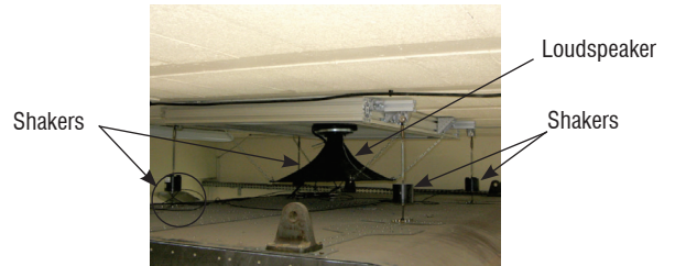
Figure 17 - Mechanical deck of an Onera cabin mock-up, with shakers and loudspeaker
