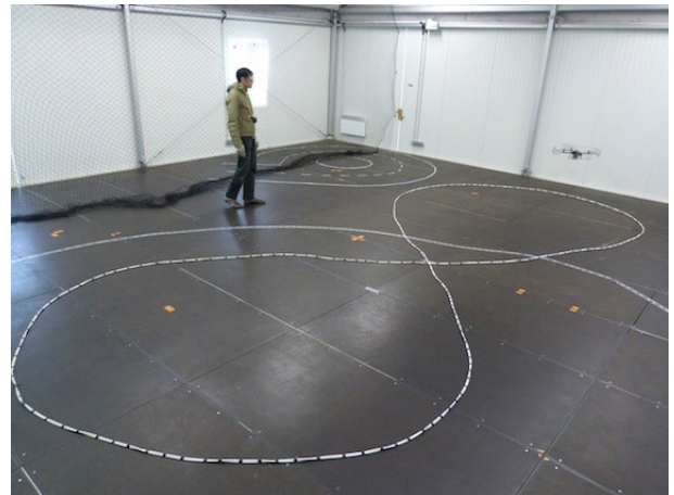
Figure 5 - Line following mission: the quadrotor flies over the line autonomously
