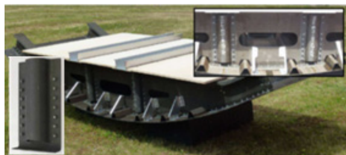
Figure 8 – Drawing of the dynamic test rig set up on the 2mx2m test floor of the ONERA crash tower (left) and picture of the AIRBUS composite crashworthy Sub-Cargo demonstrator before testing (right)
