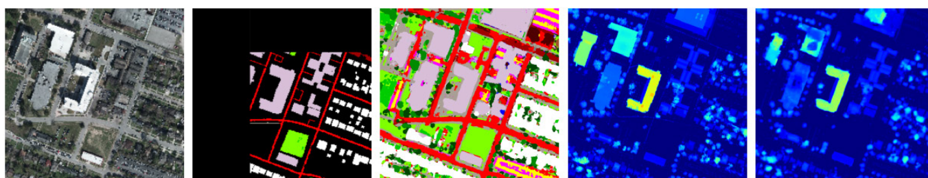
Figure 10 – From left to right, input RGB image, semantic ground-truth and prediction. Black represents no information. Height ground-truth and prediction evaluated for DFC2018 data over Houston.
