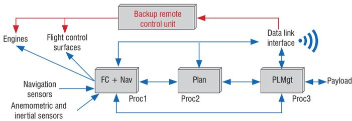
Figure 1 – Typical UAV 1<sup>st</sup>-generation architecture
