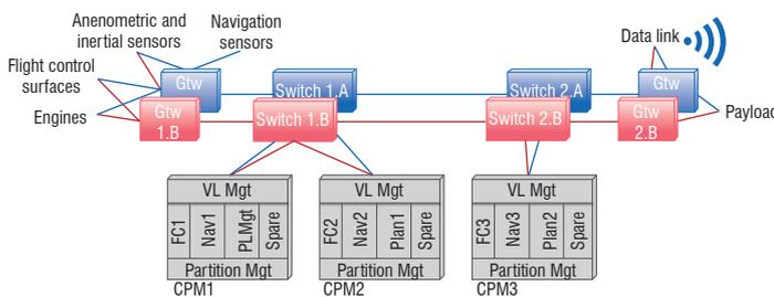
Figure 2 – Example of UAS IMA architecture
