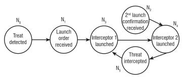
Figure 13 - Example of Bayesian Network used to model a threat interception by two interceptors
