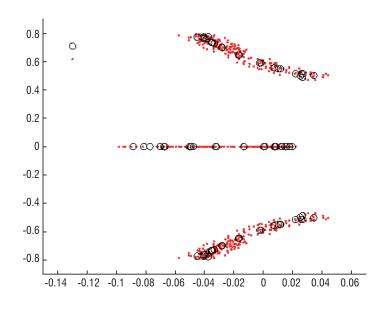
Figure 8 - Pole dispersions for Dutch Roll and Spiral stability modes Comparison between Monte-Carlo and PCT
