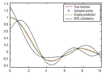
Figure 4 Kriging interpolation with 5 sample points
