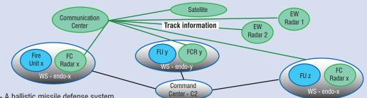
Figure B3 - 1- A ballistic missile defense system
