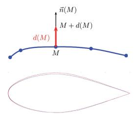
Figure 1 - Geometrical design defaults of an airfoil on the pressure distribution
