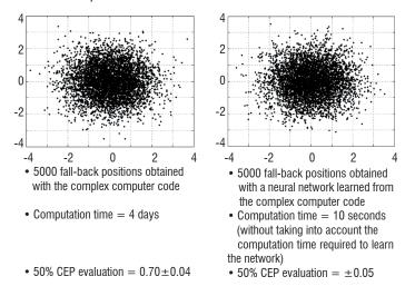
Figure 3 - Fall-back zone estimation of a space launcher stage
