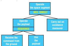
Figure 14 - A tree reflecting the (partial) behavior of a space system
