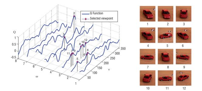
Figure 5 - Active recognition of car type from a database. For each class, the Q-function that determines the angle under which an agent should inspect a vehicle for better recognition has been obtained by Kriging and EGO
