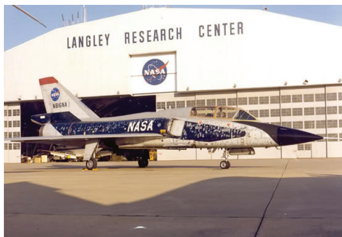
Figure 3 – NASA F-106 B research aircraft. [Photo NASA]. The aircraft was devoted to the NASA Langley Research Center from 1979 to 1991. Modified for in flight lightning experiments in 1979, it was used by NASA for in-flight lightning experiments from 1980 to 1986
