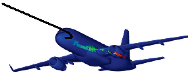
Figure 17 - Result of a sweeping starting from the initial attachment point and sweeping along the fuselage. The color scale represents the location in time of the attachment point on the fuselage. The computation has been performed on a generic single-aisle aircraft in cruise flight at a velocity of 250 m/s.
