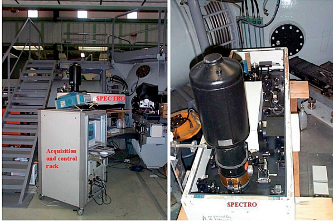
Figure 4 - Typical DLAS set up in the F4 wind tunnel. The laser emission bench and the optical detection setup are outside the vacuum chamber. The laser beam enters the vacuum chamber through \text{CaF}_2 windows and crosses the flow at the smallest possible angle to the flow's axis, so as to induce the largest Doppler shift for velocity measurement purposes.
