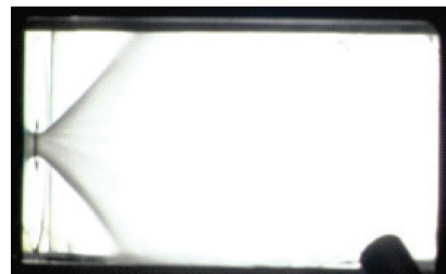
Figure 21 – Hollow cone spray produced by a swirl injector (without combustion, LOX side alone)
