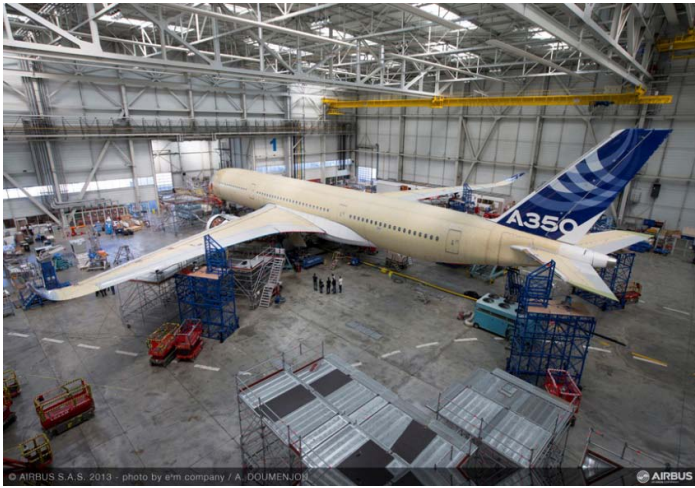
Figure 25 - GVT campaign of the A350 XWB-900 in Airbus facilities (Toulouse, France)
