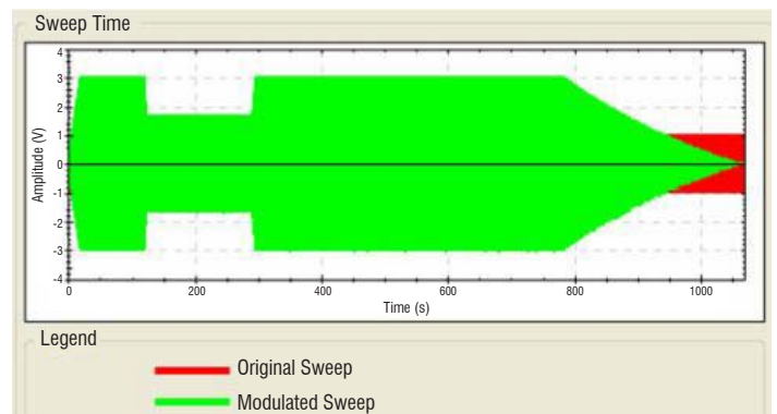
Figure 19 - Maximizing the force level over frequencies and example of a modulated excitation time signal
