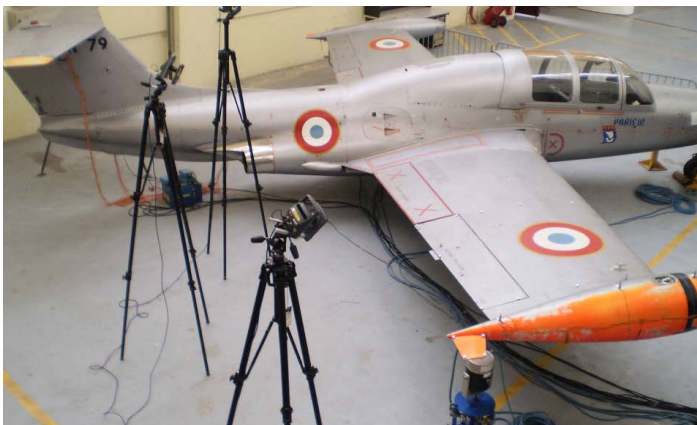
Figure 31 - Photogrammetry on the "Paris" aircraft at ONERA (S1Ch, Meudon)
