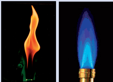
Figure B1-1 - Examples of diffusion flame (left) and premixed flame (right)
