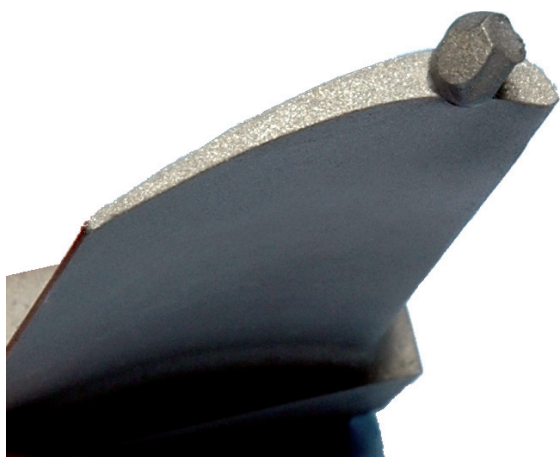
Figure 6 – Investment cast Nb-Si based demo blade (height ~ 120 mm) [2]
