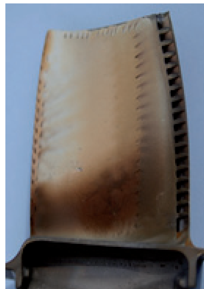
Figure 9 – After service high pressure turbine blade: pressure side covered by CMAS brownish deposit
