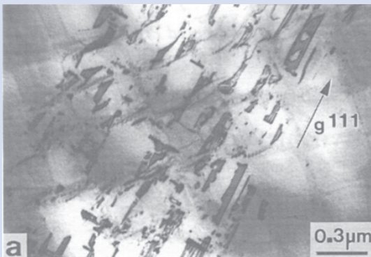
Figure B3-02 – Dislocation structures in tensile MC2 <001> SC specimens strained to 2% at room temperature: a) unaged material, b) aged material.
