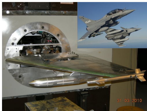
Figure 24 – Wind-tunnel validation of non-linear aeroelastic methodologies in the presence of mechanical free-plays (instability regions + LCO)
