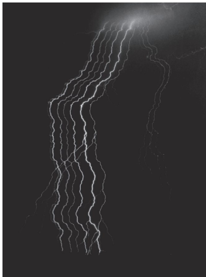
Figure 4 - Illustration of current cutoff in the channel to ground in a multi-stroke lightning flash [31]. Note the reproducibility of the fine structure of the channel tortuosity from stroke to stroke.
