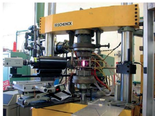
Figure 13 – Perforated tubular specimen (left) and the high temperature tension/torsion/internal pressure experimental device (right)
