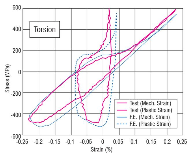
Figure 9 – Stabilized mechanical stress-strain behavior of <001>-oriented single crystal superalloy AM1 under axial-torsional Thermo-Mechanical Fatigue (TMF cycle defined in figure 7)
