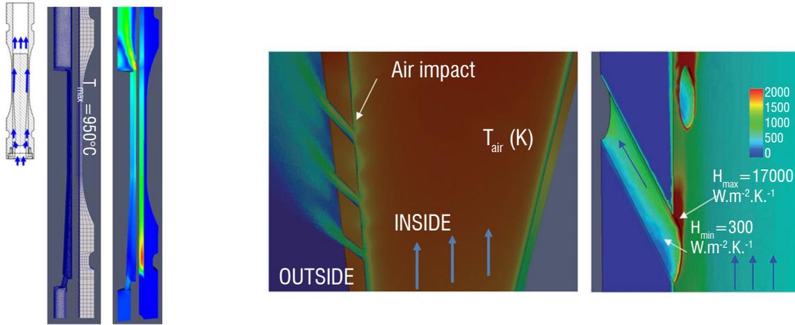
Figure 14 – Thermal/Solid/Fluid coupled calculation: smooth specimen (left) and perforated specimen (right). Temperature contours and the convective heat transfer coefficient  $h$  governed by the fluid velocity
