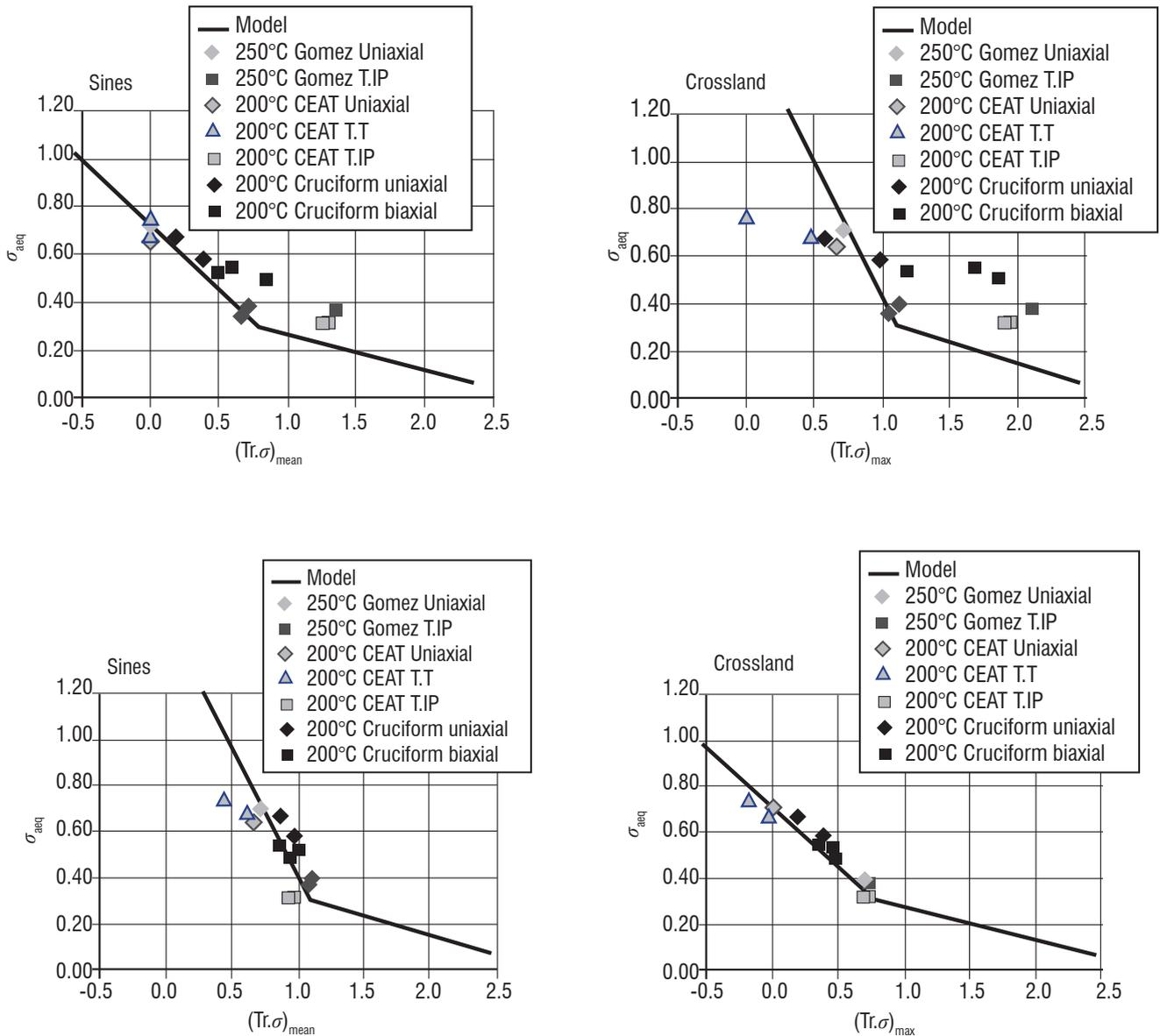
Figure 12 – Comparison of Sines, Crossland, Gonçalves and the ONERA criteria on Ti64 superalloy
