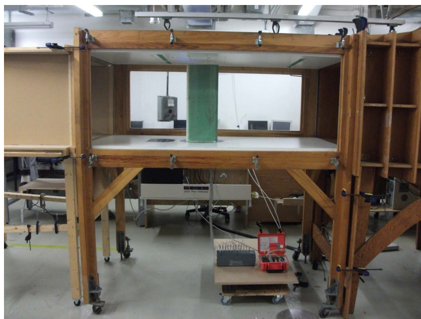
Figure 9 – Installation of the model in the wind tunnel
